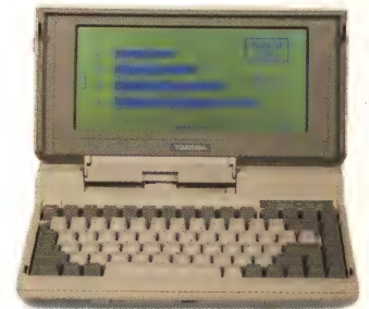
T1200FB: 9.8 pounds, 9.54MHz 80C86, 1MB RAM. 2 720KB 3 1/2" floppy drives, removable/rechargeable battery pack.
